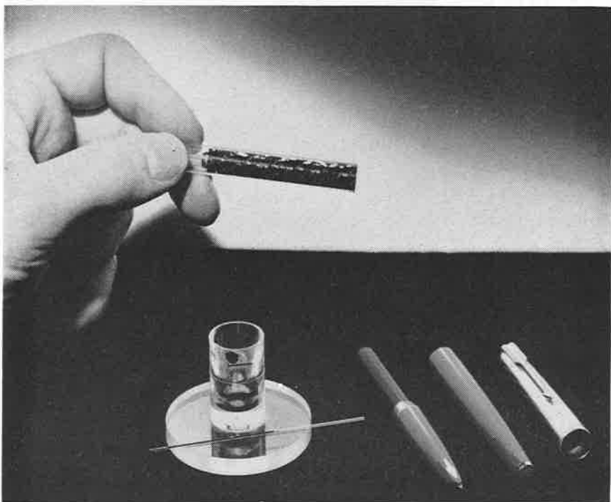
A demonstration capillary cell begins to fill and seconds later has emptied the vial.
